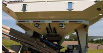
WINDOWS AND LIGHTS FOR DETERMINING FILL LEVEL
