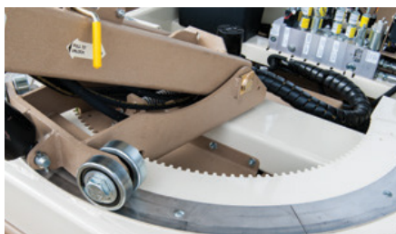
TURNTABLE FEATURES 3/4" INCREMENTS
