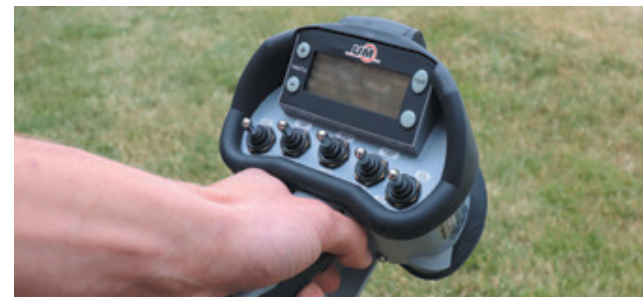
7-FUNCTION HANDHELD WIRELESS REMOTE
